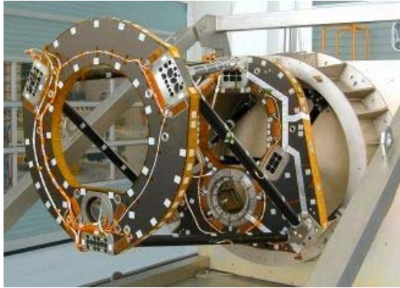
Fig. 19: Mechanical part of the afocal (Alcatel): aluminum honeycomb sandwich plates, carbon truss, titanium insert for the camera, heater lines.
