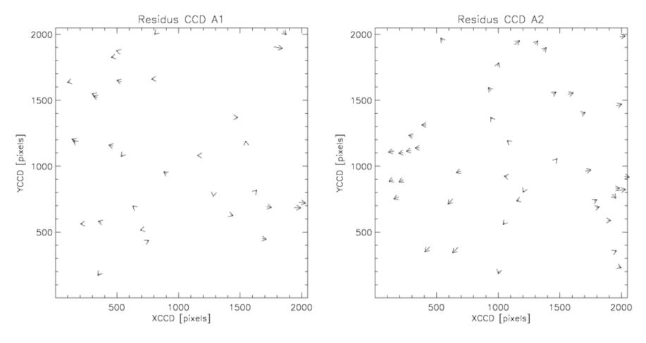
76 stars - residuals mean 4.0 mic max 9.5 mic (with theoretical Zemax distortion model)
