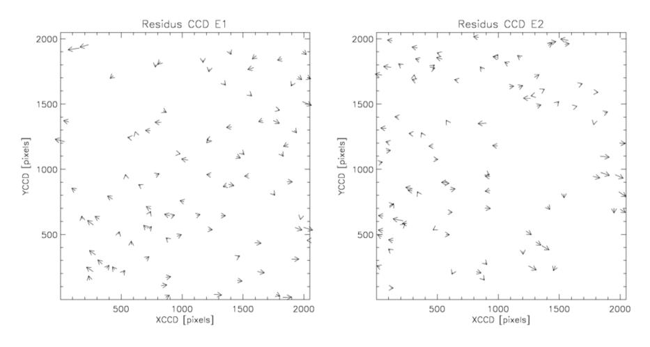
about 200 stars - residuals mean 4.6 mic max 14.6 mic (with theoretical Zemax distortion model) I←
