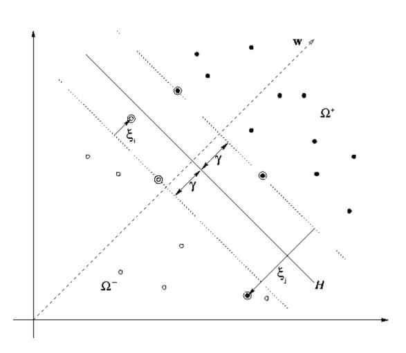
Support Vector Machines try to find the optimal separating hyperplane following the Structural Risk Minimization principle.
