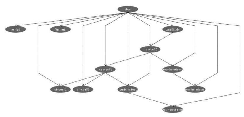
Bayes net constructed using the K2 search algorithm and metrics (although alternative metrics were tried such as MDL, AIC and entropy alone). Conditional probability distribution was computed with a maximum likelihood estimator.
